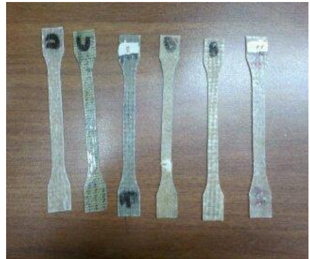
Figure 3: samples of tensile test at ASTM-D638 [Experimental work P39]
